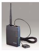
integrated cellular data module,. This enables the dispatch to track the vehicle or even take manual or automatic action. The potential of this technology is tremendous.
