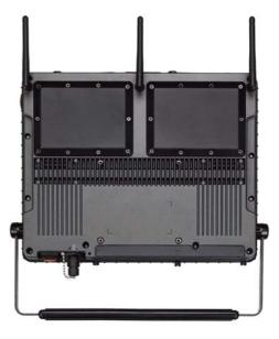
There are three external antenna connectors. Since the radios are located inside the sturdy metal case, stub antennas are necessary for best wireless reception.
