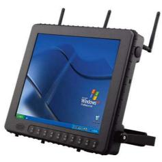
Windows XP Embedded on Flash or as a full Windows XP machine using a hard disk. Should the application demand it, DT Research can also configure the machine with Linux. Our review unit felt very quick and responsive running XP Embedded on 2GB of Flash and an efficient 1GHz AMD Mobile Sempron processor. Since there is no fan, the Web-DT 520 runs in complete silence. The enclosure is sealed to IP65 specifications and has been tested in accordance with MIL-STED-810F for shock, vibration and
