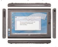
For expansion, the J3500 has a single Express Card 34 slot and an optional Smart Card slot. With space at a premium and both USB and Express Card SD adapters, Motion decided to forego a separate SD slot. A SIM card slot can be found under one of the batteries.
