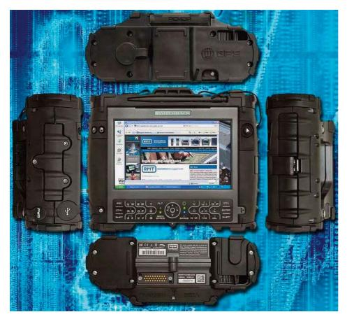
by three Allen screws as well as the DC power input and a USB 2.0 port, both with the protected rubber plugs in place. The plugs are screwed onto the computer and can easily be replaced. The hard drive in our review unit was an 80GB Toshiba 1.8-inch MK8009GAH unit spinning at 4,200 rpm.
